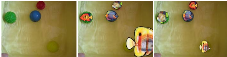
Figure 5: Original Frame (left); When Normalized RGB Goes wrong (center); HSV processing (right)
