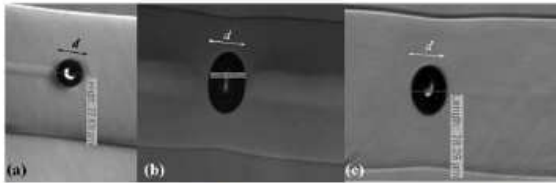
Fig. 2. Micrographs of some cavities. (a) The PCF is not pressurized, (b) and (c) the pressure was 1.5 bars and 1.0 bar, respectively. d refers to cavity length. The fiber used was the PCF-B.
