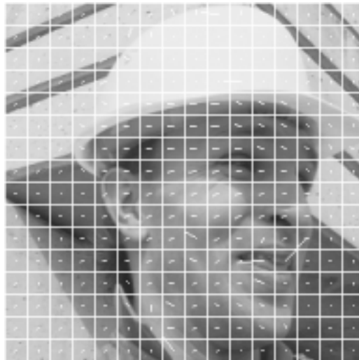
Figure 7. Motion Vectors in a Video Frame
