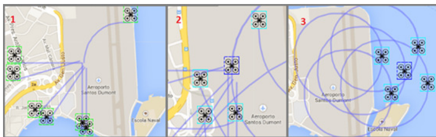
Figure 14 - Control Interface: (1) Shows six UAV flying in FREE status, patrolling around; (2) Shows four Slave UAV surrounding a central Leader before the swarm be in correct formation and (3) Shows a swarm correctly flying around.
