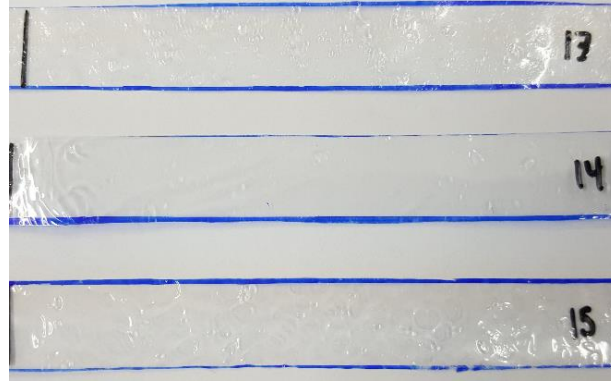
Figure 4.4. PVA film for mechanical test
