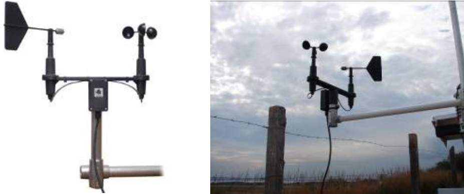
Figura 4-7 Anemômetro e Cata-Ventos Wind Sentry3002-5 (Young Meteorological Instruments).
