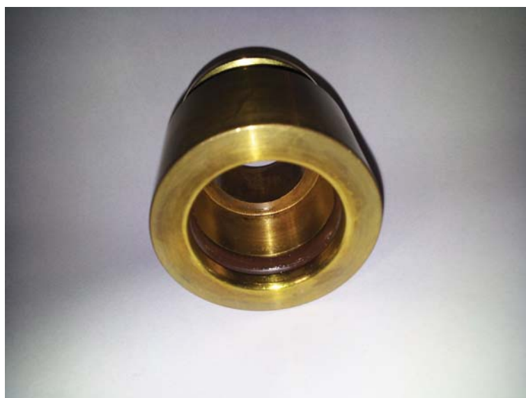
Figure 3.6: Adapter and the o-ring that seals the quartz tube.
