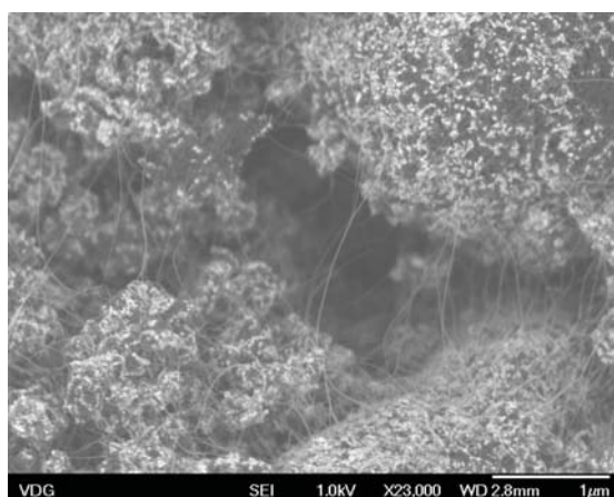
Figure 5.2: SEM images of a reference sample produced using Ethanol at 850°C. This temperature gives the highest amount of produced tubes for this precursor.
